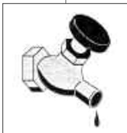
*Assuming that nothing is on in the house, the water at the bibb is a combination tank water and pump water, both being restricted by house piping. It tells you nothing about recovery.*
